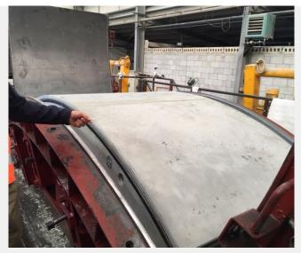
The monofilament micro synthetic fibre is added at the specified dosage during the fully automated batching process, before the concrete mix is placed and compacted into the tunnel segment moulds at the Precast Facility.
