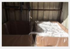
Monofilament Micro Synthetic Fibre Provides passive fire resistance to reduce explosive spalling of the concrete tunnel lining in the event of a fire. A continuous length of fibre is cut to specified length during the production process before addition to the concrete mix.
