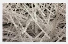
Macro Synthetic Fibre DURUS \$400 Dosage of 4kg/m³ to provide protection from shrinkage cracking and enhance the durability of the 100mm screed topping.
