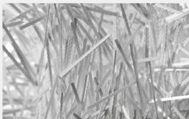
**DURUS Macro Synthetic Fibres -** Macro fibre made out of polypropylene. Improves the bond with the concrete.
