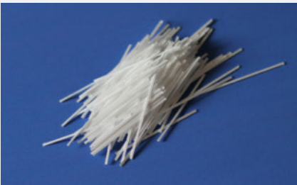
Durus S400 BS EN 14889 Class 2 Embossed Macro Fibre at 4 kg per cubic metre of concrete.
