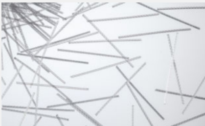
Durus S400 BS EN 14889 Class 2 Embossed Macro Fibre at 4 kg/m 3 of concrete
