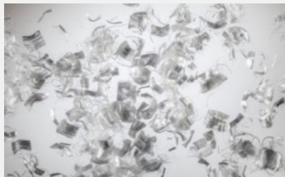
Fibrin XT BS EN 14889 Class 1a Micro Monofilament Fibre at 0.910 kg/m 3 of concrete
