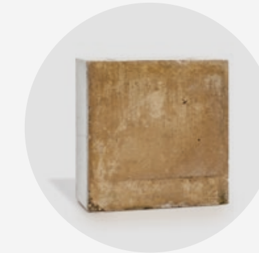
BRE sample with Ignis subjected to European Hydrocarbon Curve showing no spalling
