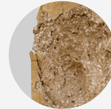
BRE sample without Ignis subjected to European Hydrocarbon Curve showing severe spalling
