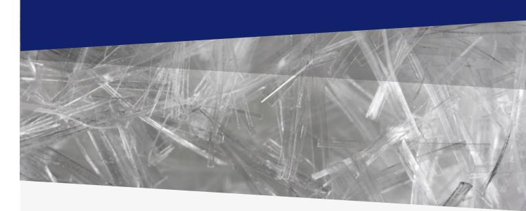
The Crackstop range of fibrillated polypropylene fibres reduce the occurrence of plastic shrinkage cracking and plastic settlement, whilst enhancing the surface properties and the durability of the hardened cementitious product. The fibres are cut to lengths of 3, 6, 12 or 18 mm and have a nominal thickness of 50 microns. Crackstop fibres are coated with surfactant to improve dispersion and bond.
