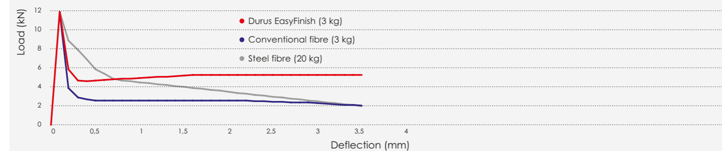
Fig. 4 / Three-point flexural bending test according to EN 14651
