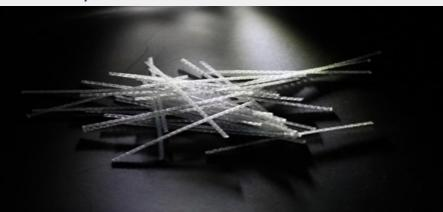
Effective replacement of conventional steel mesh reinforcement in marine concrete applications.
