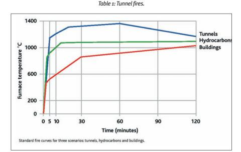
Figure 3: Standard fire curves for three scenarios: tunnels, hydrocarbons and buildings.
