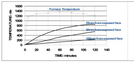
Figure 4: Typical temperature profile within concrete during test.
