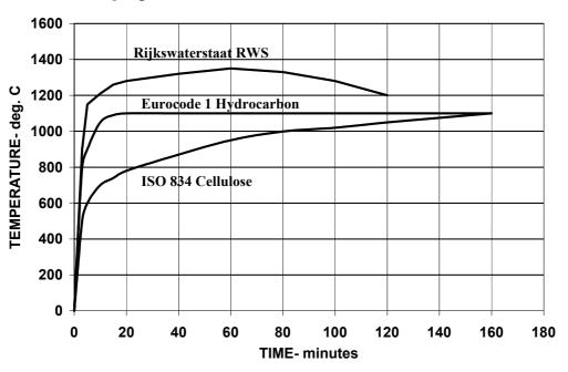
Fig 1. \_STANDARD FIRE CURVES USED IN CTRL TESTS
