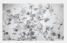
Fibrin XT Micro fibre made out of polypropylene. Reduces plastic shrinkage.
