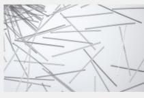
DURUS \$400 Macro fibre made out of polypropylene. Improves the bond with the concrete.
